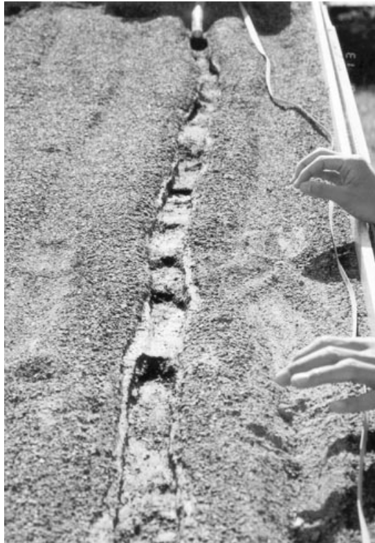
FIGURE 3. View of experimental cyclic steps produced by Koyama & Ikeda (1998). The width of the channel is approximately 5 cm; the average slope angle is 6^\circ .
